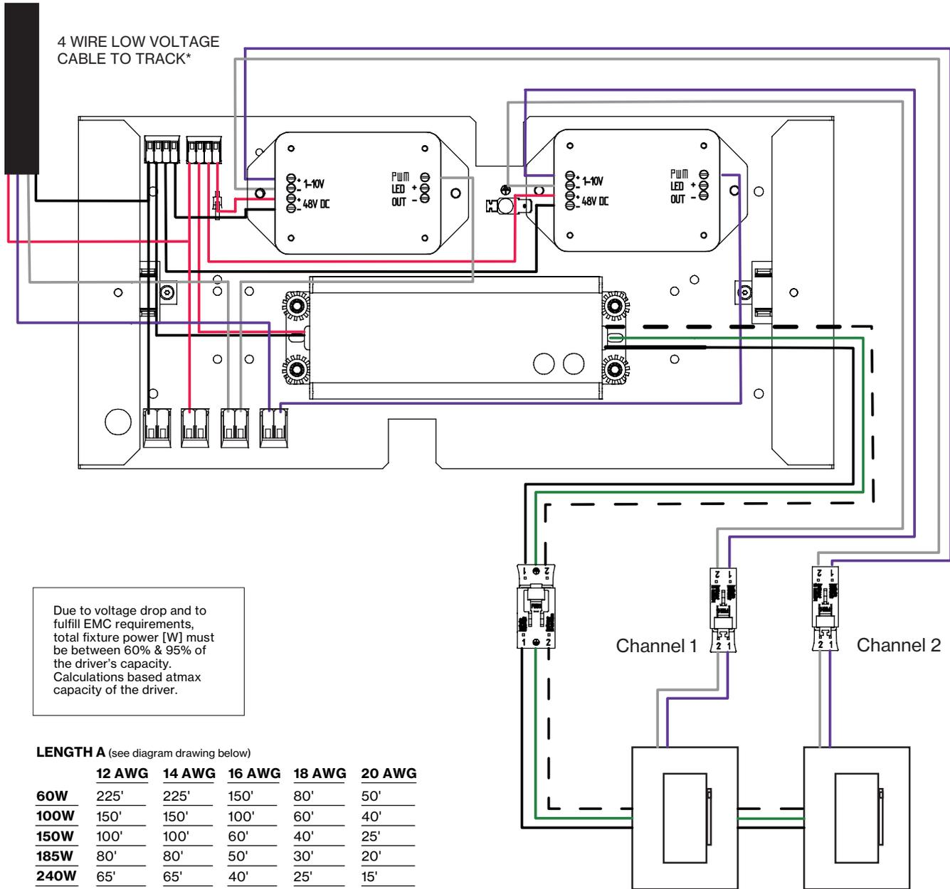
Due to voltage drop and to fulfill EMC requirements, total fixture power [W] must be between 60% & 95% of the driver's capacity. Calculations based at max capacity of the driver.
