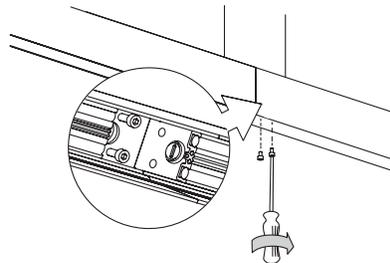
22 A. **Track 1.1:** Turn tensioning screw clockwise
