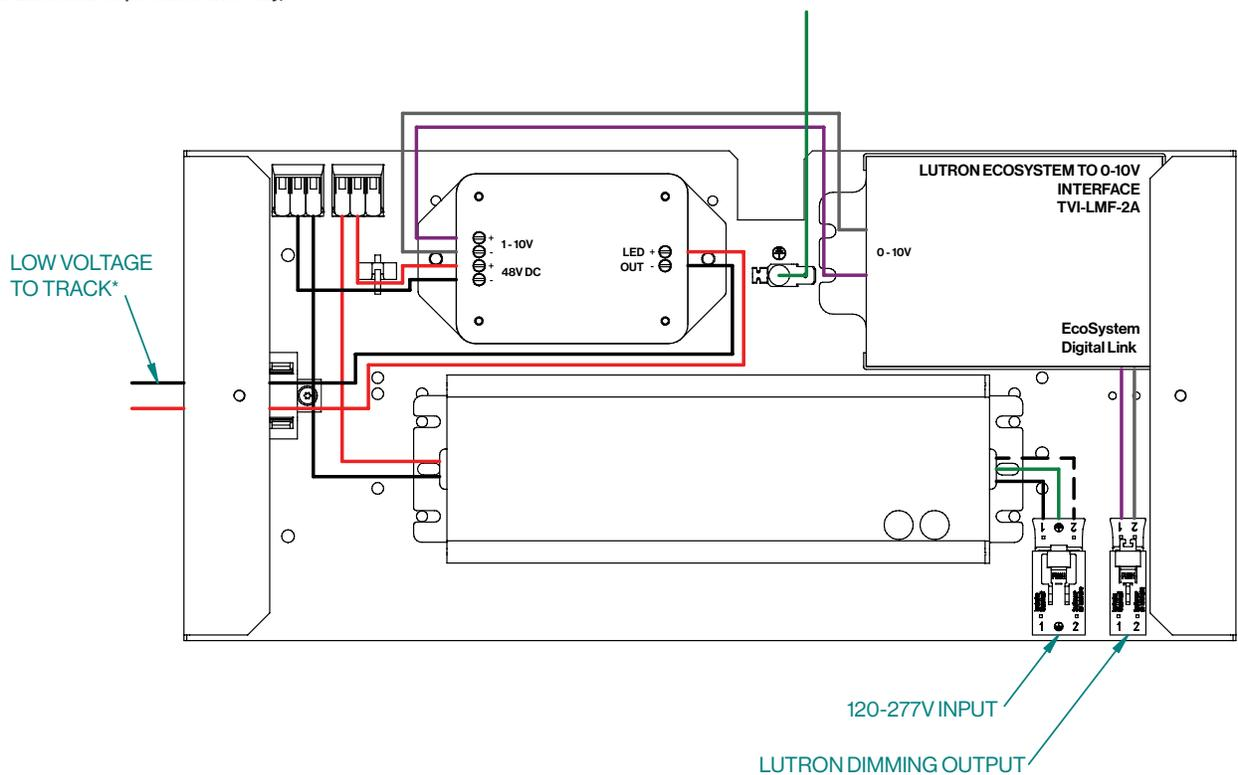
\*Please check distance limits (voltage drop table) - any cables in the plenum space (including low voltage > 100W) need to be in conduit
