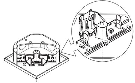
15. Secure power feed cable to suspension, cable every 3 inches using cable ties (cable ties provided by others)
