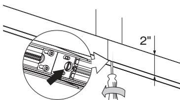
23. **Insert T-Connector (optional):** Use screws to attach T-connection
