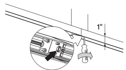
22 B. **Track 1.2:** Turn tensioning screw counter-clockwise. Repeat steps 18-22 for additional channels
