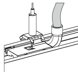
26. Align the indirect connector with the linear connector from above
