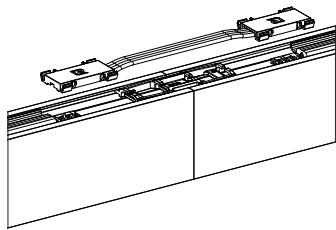
27. Snap the indirect connector to the linear connector. Follow steps 22 and 23 to complete installation.
