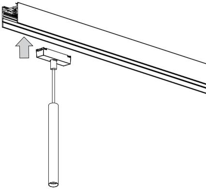
**TUBE:** At the appropriate length, TUBE can be installed between M-LINE tracks
